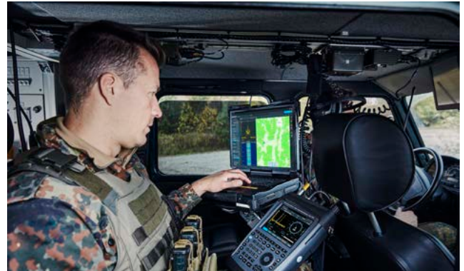
Picture 4: The ability to dismount the EW CESM sensor from the tactical vehicle enables the mission to be carried out on foot. (Source: Rohde & Schwarz)
